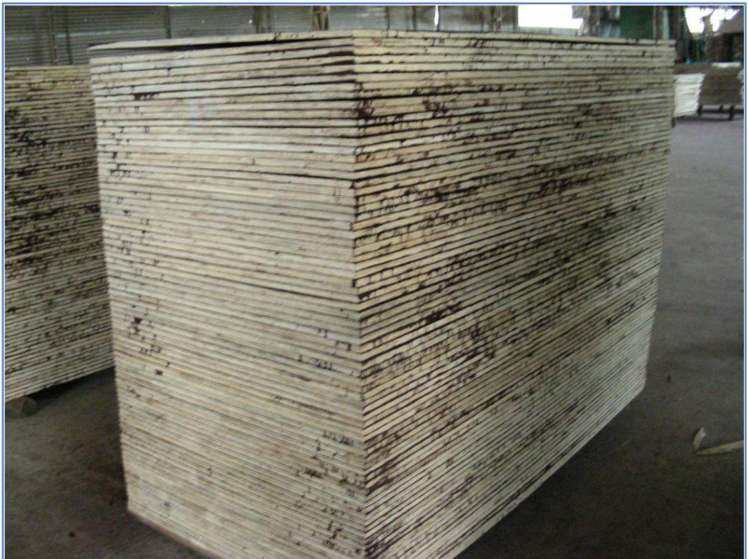
Photo 4-10: Plywood sheets at plywood factory to where the veneer sheets (in Photo 4-9) are transported for secondary processing.
