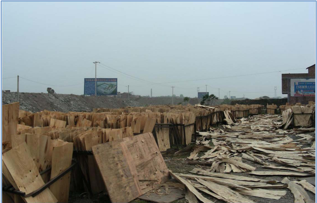
Photo 4-9: Veneer sheets having been peeled on the lathe (Photo 4-8) and sliced , drying in open air.
