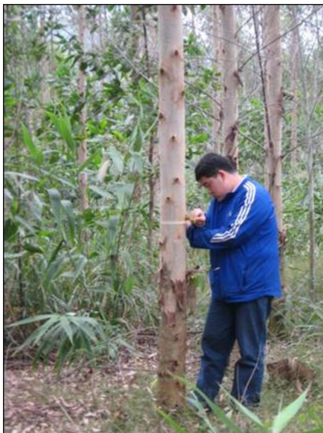
Photo 2-1: Measurement of Plot-tree Diameter at Breast Height (1.3 m)
